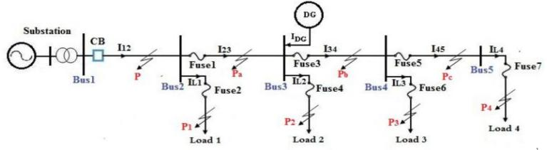
For coordination between Fuse 3 and Fuse 6, Fuse 6 should operate before Fuse 3; this requires that Total Clearing (TC) time curve of Fuse 6 is below the Minimum Melting (MM) time characteristic of Fuse 3 by a safe margin for any fault at position P3. As shown in Figure the fuses are coordinated for all fault currents below IFmax. After installing DG, (IF3= IF6= IFault = Is+ IDG2), it is possible that the fault current level exceeds IFmax and the coordination between these two fuses is lost
